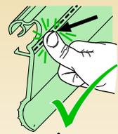
Push along line as shown to lock. **DO NOT** push on soft area!
