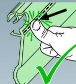
Push along line as shown to lock. **DO NOT** push on soft area!
