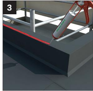
Apply a generous, continuous bead of silicone to the outer perimeter of the top surface of the kerb.
