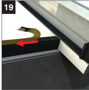
Peel back a small tab of the protective film on the glazing support from the eaves.
