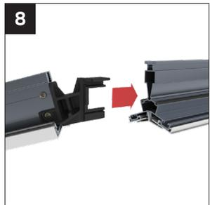
Prop the ridge body, now attach the left hand hip rafter by inserting the ridgeLOCK into the ridge body. The branding 'ridgeLOCK L20' indicates this is a left hand part.
