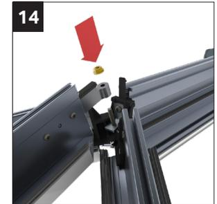
**If the project contains central rafters between the hips.** Position the rafter between the two hip rafters, secure using the 30mm hex bolt and flanged nut provided.
