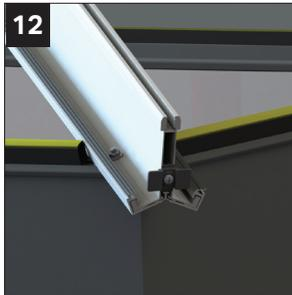
Remove nuts on eaves beam. Fit hip rafters onto bolts at eaves end and hand tighten nuts.
