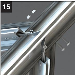
**If the project contains jack rafters:** Offer up the jack rafter to the hip at the ridge and push the bolts through the jack rafter bracket and secure with flanged nuts.
