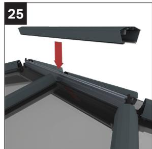
Fit the ridge top cap, ensure that the top cap clips are evenly spaced. Push down along the length to check the top cap is fully engaged.
