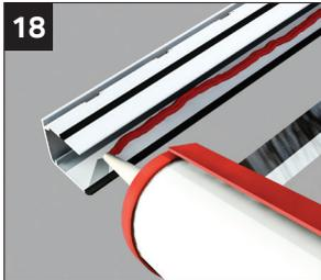
MS Polymer sealant only on Self cleaning glass
