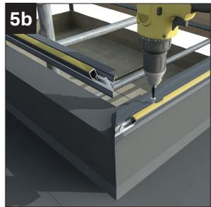
Check the required number of bolts are in the eaves beam/rail. Seal cut ends of eaves. Line up eaves along outer edge of kerb\* and screw down using appropriate 5mm x 50mm fixings (not supplied) ensuring good engagement. \*As shown in previous image.
