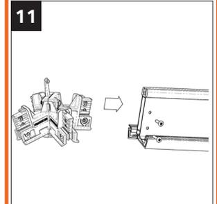
Fit each hip rafter to the tenons of the ridgeLOCK. Secure in place into pre drilled holes using M5 x 16mm screw in the upper hole and the M5 x 20mm screw in the lower hole.
