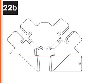
Cut the ends off two weathering shields. Ensure glass is clean and dry before fitting. Peel back protective film from shields and position (adhesive face down) on glass, locating around the ridgeLOCK and hip rafters.
