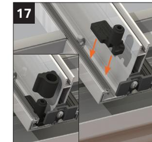
Snap off appropriate handed glazing stop. Place this onto the base of the glazing rafter. Snap off a gromet from the kit, this will slot over the up-stand on the glazing stop. Repeat this for all glazing rafters on the roof. DO NOT screw in place until step 21.
