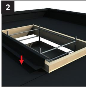
Wrap the membrane up the kerb and lap over the top of the kerb ensuring that a watertight finish is achieved.
