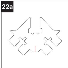
If the project contains central rafters between the hips. Perform the cut detailed in the image above approximately 15mm in length.
