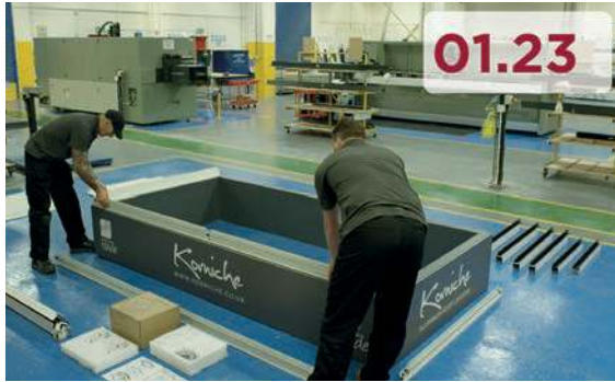
CORNER BRACKETS TO EAVES BEAM
